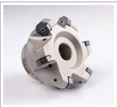
AFM45-XN07 face milling cutter with heptagon inserts, 14 cutting edges, with nanostructured PVD coating. Used in rough milling the flange face, with a high performance/cost ratio.
