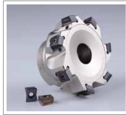
ASM90-LN13 square shoulder milling cutter with tangential mounted inserts. The insert has 4 cutting edges, can be used to machine the boss surface on the turbocharger.
